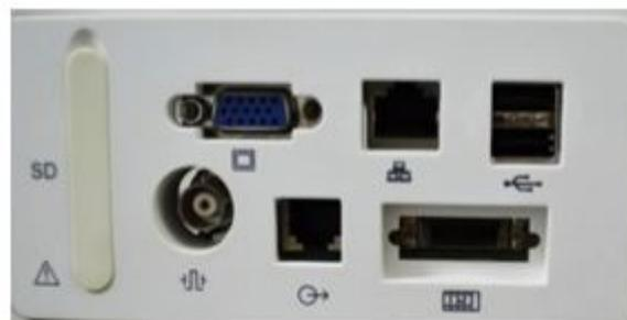
Figura 5 - Conectores do Monitor LiFEtouch M10
