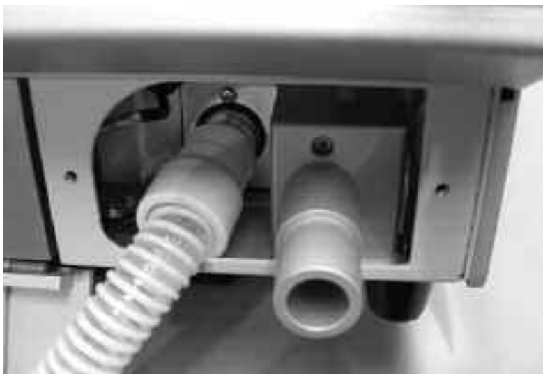
Figure 4-19 Use circuit to loosen Oxygen Sensor
